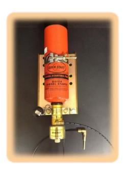
Attach Tubing to the Control Fitting with the Compression Nut & Ferrule & a 3/8" wrench. Pull tubing to ensure the connection to the compression fitting is tight. Suggested torque spec: 25 In/Lbs.
