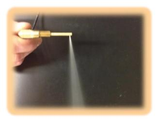
Perform Functional Spray Test by activating the system with the atomizer out of the port. Ensure you clear a space in front of where the ether is going to be atomized. Ensure atomization/vaporization. Spray should look like the picture.
